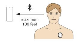
Before pairing, make sure you've enabled Bluetooth on your phone. The sensor must be within Bluetooth range of your phone to receive data.
