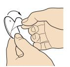
Remove plastic film from the back of the sensor.
